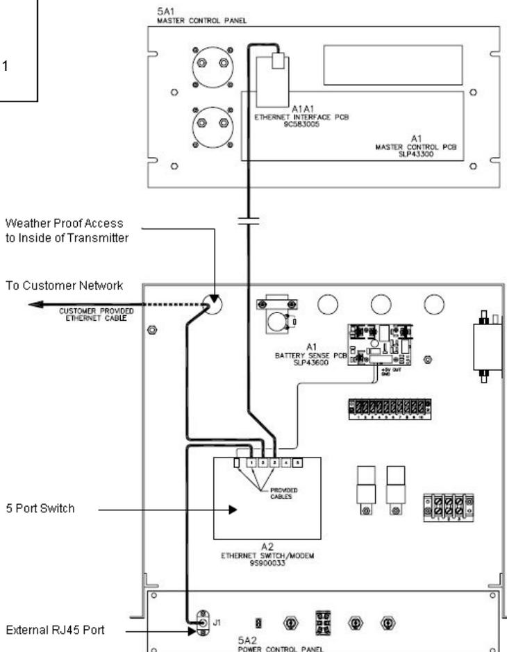
The SE125 IP66 Transmitter comes standard with an internal 5 Port Switch. There are two access points to the Switch. The first is a convenient external RJ45 port located on the front of the transmitter. The second is weather-proof access hole through the bottom of the transmitter. All 5 ports can be accessed here, once inside the unit.
